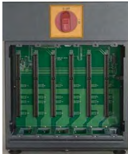
Figure 16-10 Mainframe Bay with Backplane Exposed
