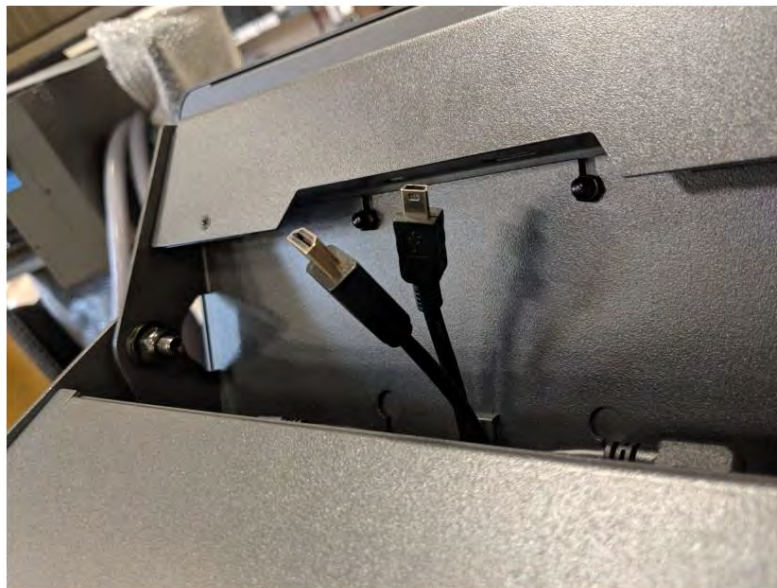
Figure 16-19 Disconnect the Mini-USB and HDMI Connectors
