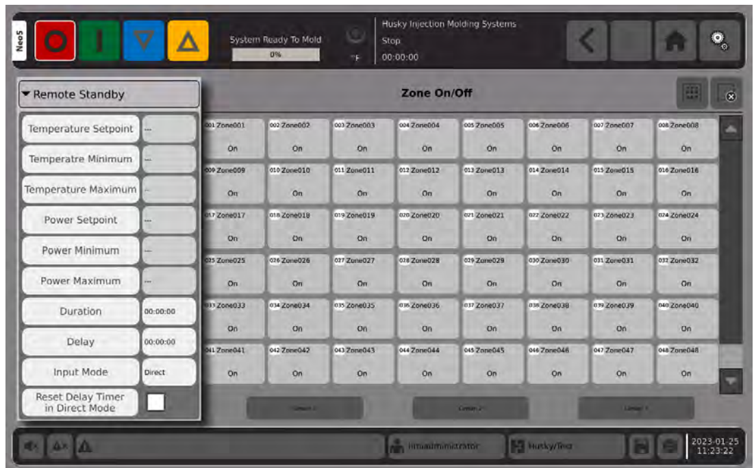
Figure 8-30 Remote Standby Fields
