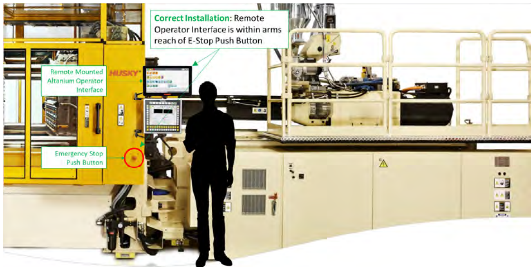
Figure 2-8 Correct Installation Position of Remote Operator Interface
