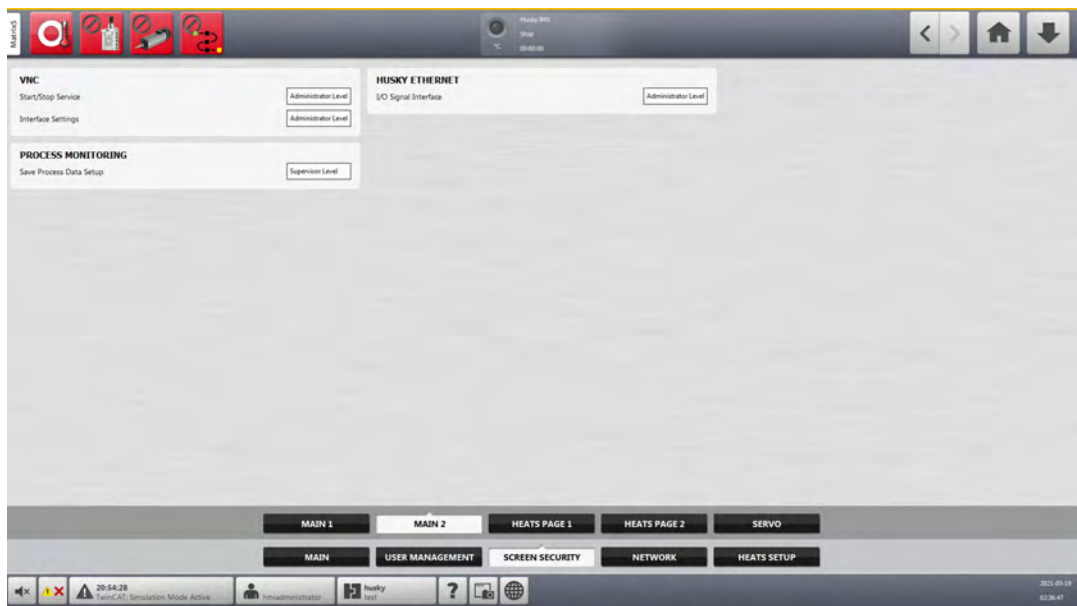
Figure 4-2 Main 2 Security Screen
