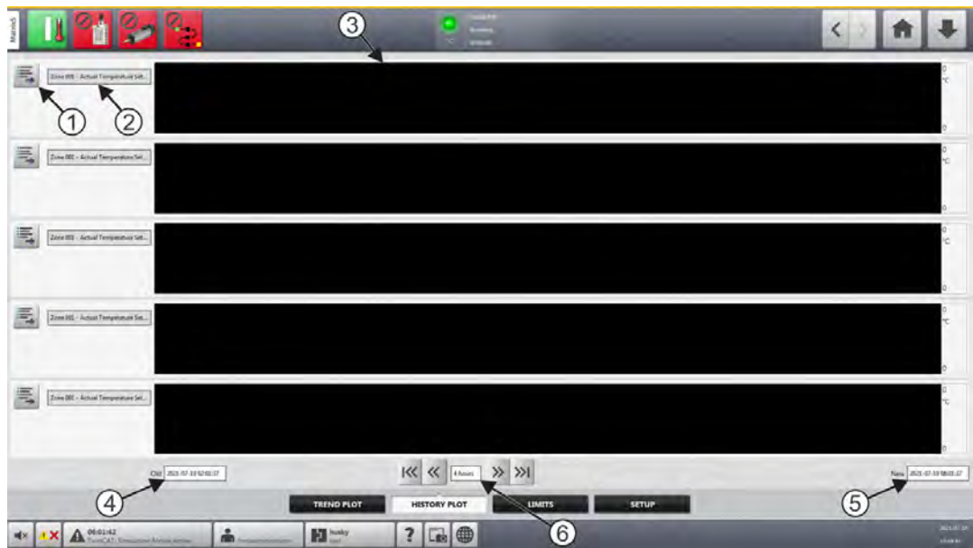
Figure 11-3 Process Monitoring History Plot Screen
