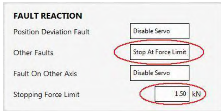
Figure 2-16 Set an Axis for a Controlled Stop
