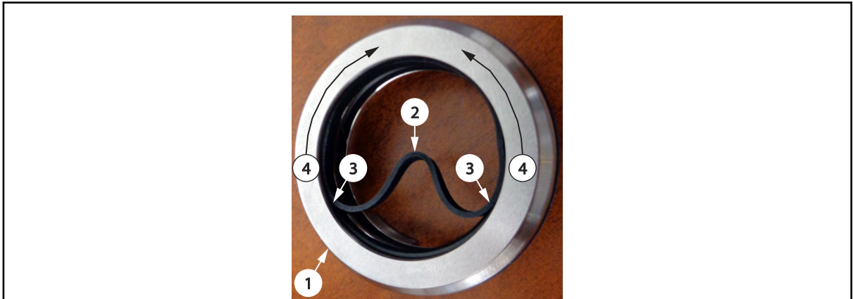
Figure 4-19: Installing the Inner Double Delta Seal Ring
