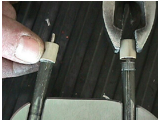
Figure 6-79: PEEK Bushing Removal and Installation
