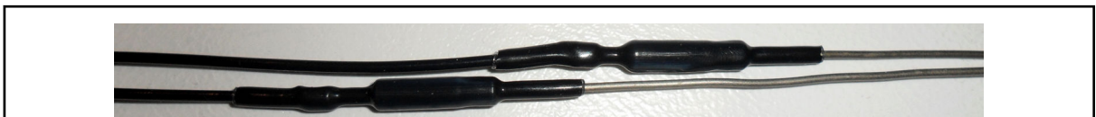
Figure 5-54: Staggering the Knuckles in the Wire Grooves
