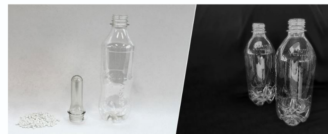
Advanced co-polyester made by Origin Materials and Husky Technologies™ using PET/F. Resin, mold, and bottle shown.
