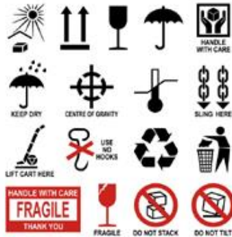
Figure 8: Package Handling Markings (DIN 55402 and ISO R 780 standards)
